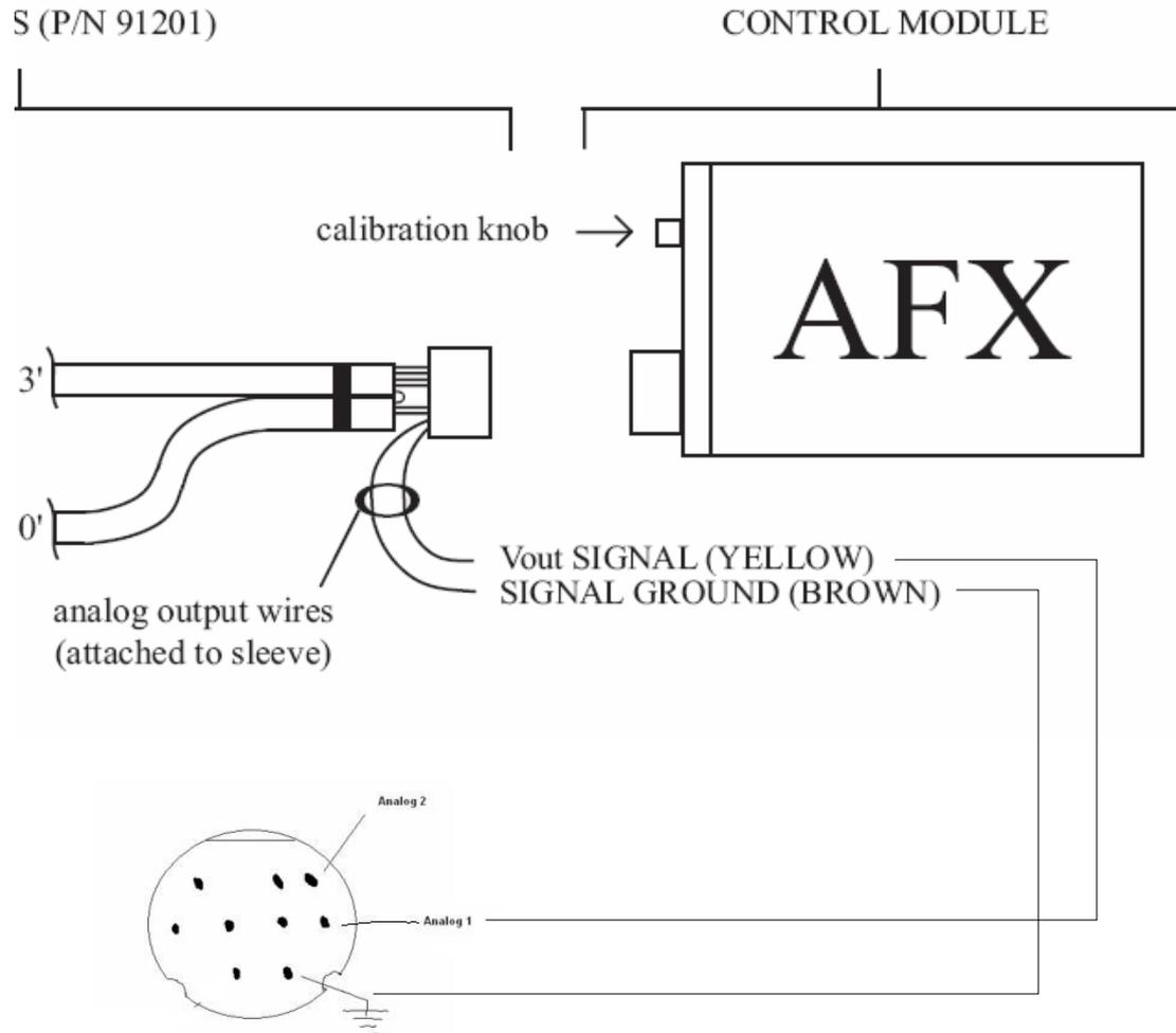
Analog input: 9 pin mini din connector, as seen from the connector side:
